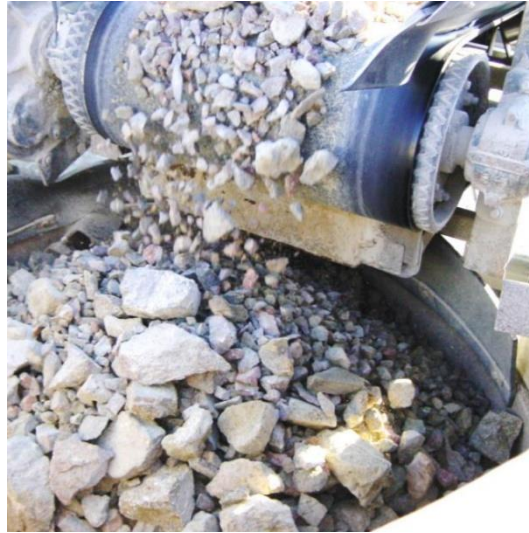
Figure 2. Typical example of size segregation in a real application
