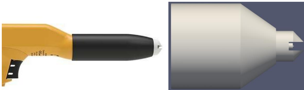
Figure 5: GEMA powder gun used for the experiments (left) and CAD model of the same gun (right)
