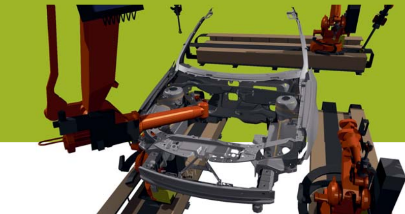
A robot is applying sealing material to a seam on the front damper in the IPS Virtual Sealing software (courtesy of SAAB Automobile AB).
