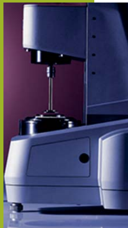
A rotational rheometer is used for characterization of the sealing material.
