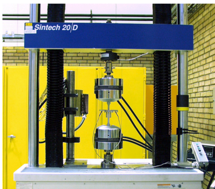
A tensile test machine for evaluating material properties, for instance the ultimate tensile strength, the yield strength, and the elongation.
