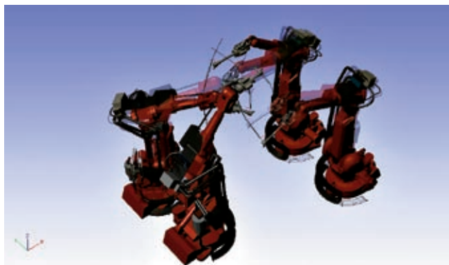
Figure 5. Where and when shall the robots wait for each other in order to avoid collisions and minimize cycle time?
