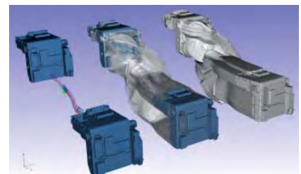
Figure 8. An assembly path and corresponding swept volume (courtesy of Volvo Car Corporation).
