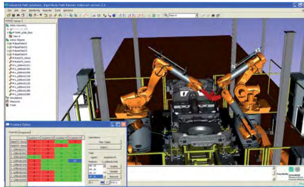
Figure 5. Task Planning. Find collision-free alternatives to perform each welding operation (courtesy of Volvo Car Corporation).
